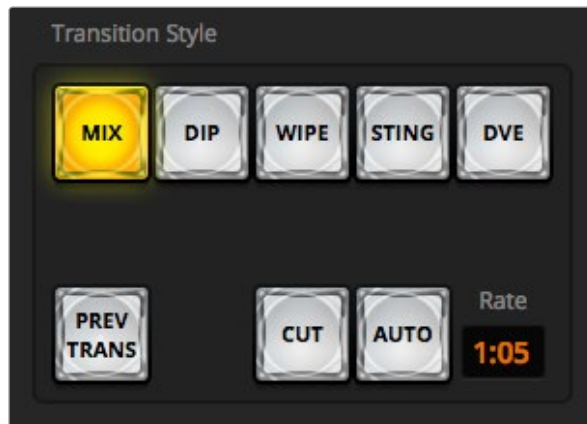
The Auto transition button is part of the Transitions Style group
