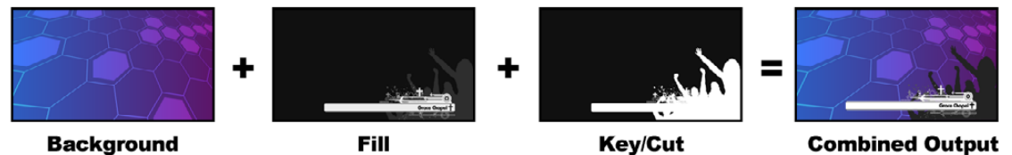
Combining a background, fill and key in a linear key
